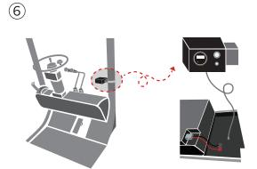
Attach the battery indicator to the cabin.
