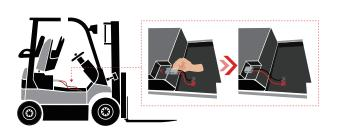
Plug in the EP Li-ion battery.
